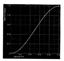
If in any experiment the length of the black part of the film increased from (say) 0.2 to 0.8 of the whole length of the cylinder, the effective length would be 0.6; and the alteration of pressure is shown by the curve to be from 0.1 to 0.9, i.e., 0.8 of the whole alteration which would be produced if a coloured film became completely black.
