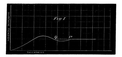
These considerations would not apply to the liquid on the thicker side of the boundary. Its surface tension being independent of the thickness, the magnitude of the latter would be indifferent.
