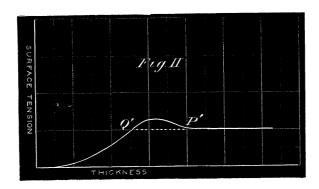
We need hardly point out that the best way of attempting to test such theories would be to measure the surface tension of a grey film. Unfortunately, however, such a film can only be obtained when the electric current is passing, and the very fact that the grey displays itself is a proof that changes in the surface are going on which may complicate the conclusions to be drawn from the experiment.
